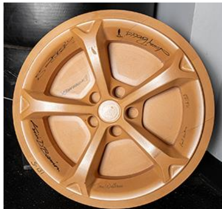
August 2022 Artifact of the Month: Signed, Three-Dimensional REN Board Representation of Corvette Wheel
