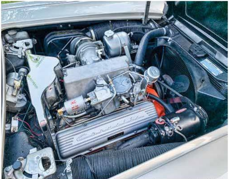
Engine has been restored and correct and original components installed
