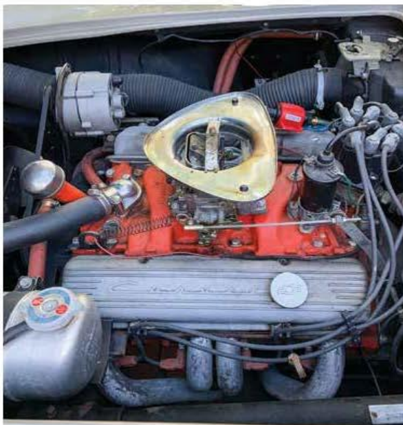
Motor that was in the car at the auction, cast-iron manifold, carburetor and headers
